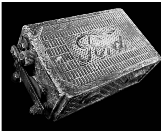
Figure 1. Magento coil from Model T Ford (~1916). The case is reportedly formulated from wheat gluten and asbestos.
